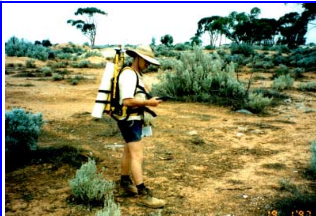
Surveying a soil geochemical grid using a Trimble AG132 DGPS unit coupled with a psion data logger in the East Yilgarn, WA.
