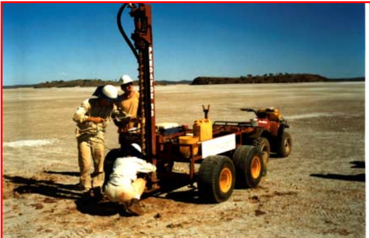
Predator 10 light weight auger on the thin salt crust at Lake Barlee, near Mt Elvire homestead, north of Southern Cross.
