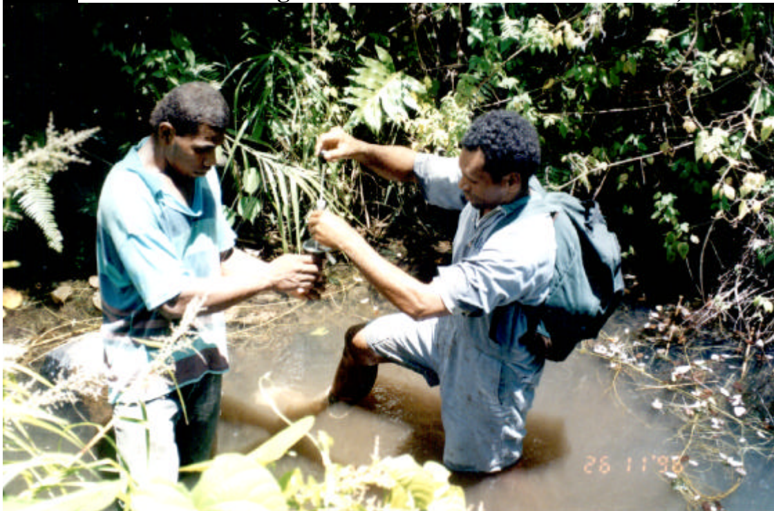
Plate 4 The sample is deposited into a geochem sample packet by pulling up the plunger and using the packet to scrape off the wet sample. “MAGSAM” is robust and can be regarded as being virtually fieldy proof.
